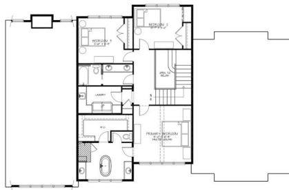
UPPER FLOOR PLAN UPPER FLOOR AREA: 1764 SQ FT * NOTE: 2'-0" OF UPPER FLOOR HALLS * * NOTE: FRAME WORKING AT 8'-0" OF IT (ALSO SEE OTHER NOTE) * * NOTE: 8'-0" OF INTERIOR DOORS (ALSO SEE OTHER NOTE) *
