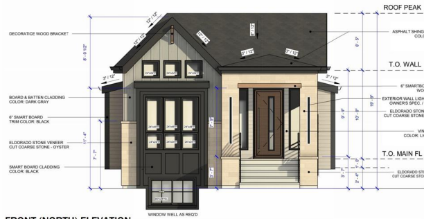
FRONT (NORTH) ELEVATION
