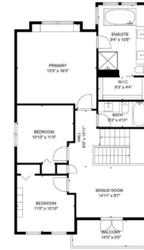
TOTAL 2870 sq. ft. Below Ground: 747 sq. ft., FLOOR 2: 884 sq. ft., FLOOR 3: 879 sq. ft. EXCLUDED AREAS: ELECTRICAL ROOM: 55 sq. ft., STORAGE: 34 sq. ft., DECK: 410 sq. ft., BALCONY: 70 sq. ft.
